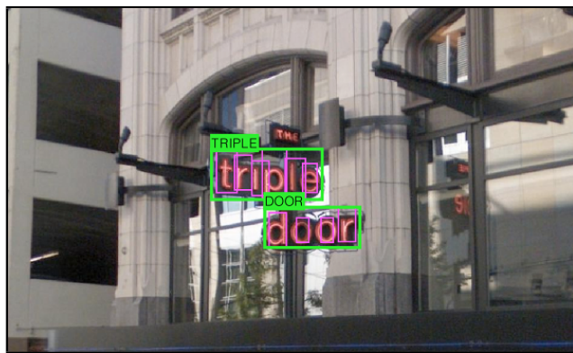
Figure 1. The problem we address in this paper is that of word detection and recognition. Input consists of an image and a list of words (e.g., in the above example the list contains around 50 total words, and include ‘TRIPLE’ and ‘DOOR’ ). The output is a set of bounding boxes labeled with words.
