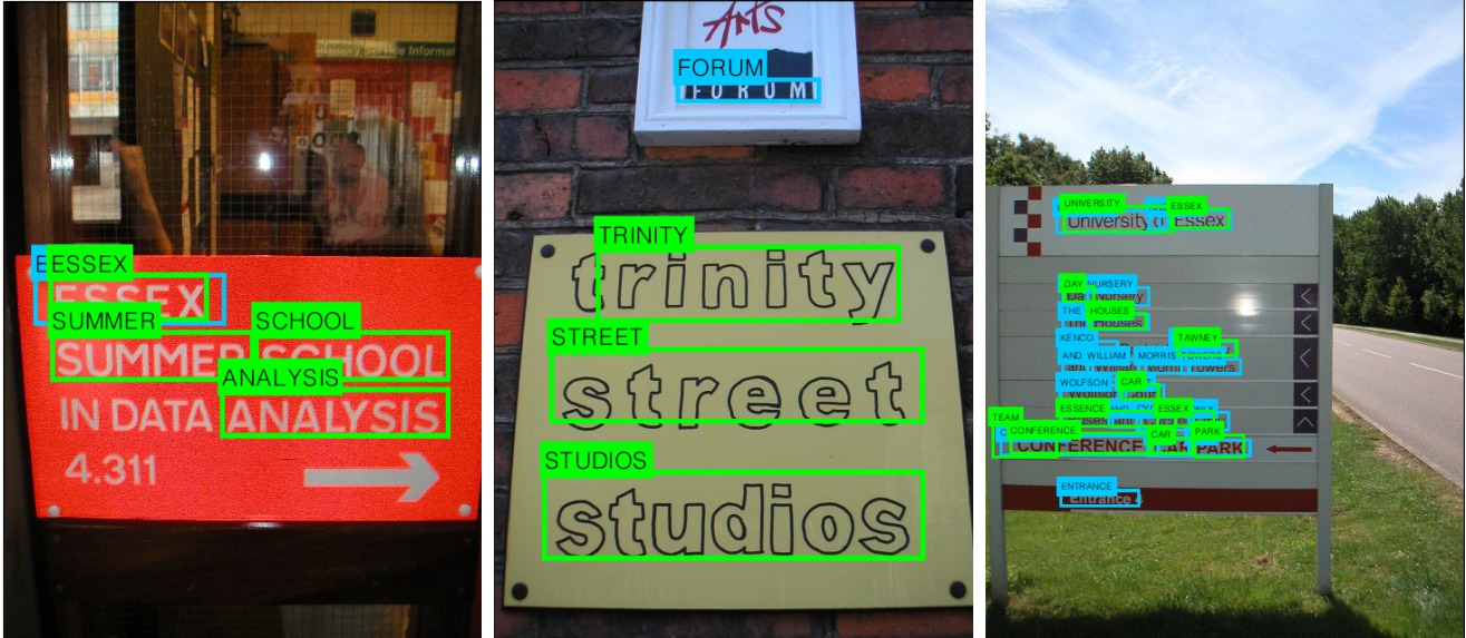
Figure 8. Selected results of end-to-end methods on the ICDAR dataset (for a lexicon with K = 20 distractors). Results from PLEX+R are shown in green and results from SWT+ABBY are shown in blue. In the first two images ABBY has trouble reading text with noisy image conditions and unusual fonts; the last image is more well suited for ABBY as it is more similar to a scanned document.
