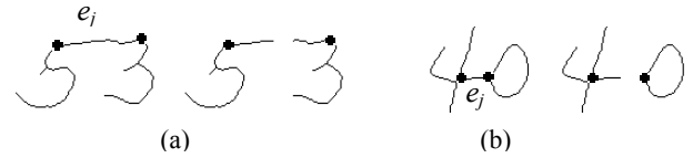
Fig. 5: Grouping of edges for single-point touches: (a) e_j is divided and grouped in both sub-graphs, (b) e_j is grouped in the left sub-graph.
