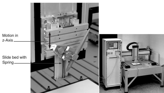
**Figure 1. Flatbed machine iselGFY44/48 with assembled pen carrier that is used in the synthesis of writing traces.**
