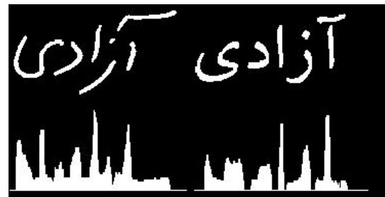
Figure 7. Valley and peak profiles of vertical projection for handwritten and machine-printed words.
