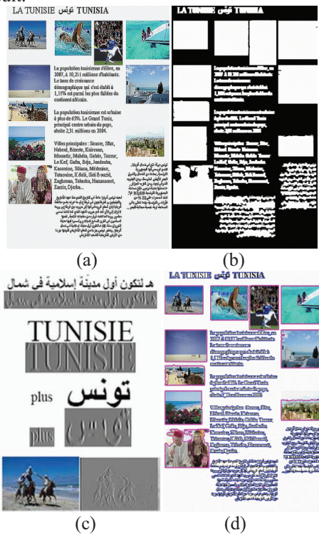
Figure 5. Segmentation process a) Input image b) Image mask c) Samples of words and images and their corresponding S.P decomposition d) Final result with Blue boundaries as text, and Magenta boundaries as non-text
