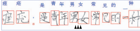
Figure 2. Example of a ground-truthed text line image in CASIA-HWDB (triangles point to a touching pair).
