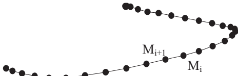
Figure 6. Variation of the horizontal and vertical intervals between the successive points of an on-line handwriting trajectory
